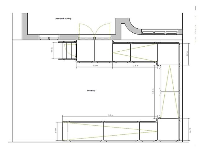
**END RESULT:** A ramp with a 1:12 gradient was installed with a few hours. It included adjustable access steps for able-bodied users.
