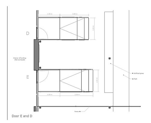
**END RESULT:** Once the new doors were in place, we installed the DDA ramps accordingly with a 1:15 gradient.
