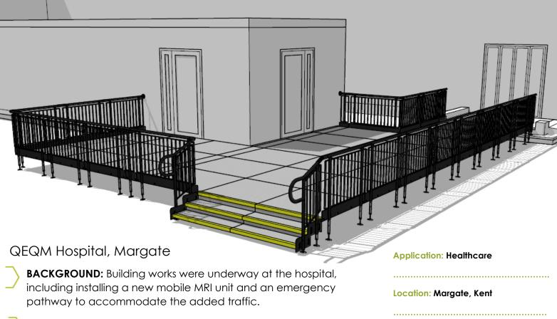
REQUIREMENT: A walkway constructed from modular platforms. The walkway would enable staff to transport patients via hospital beds to the external MRI unit for vital scans.
