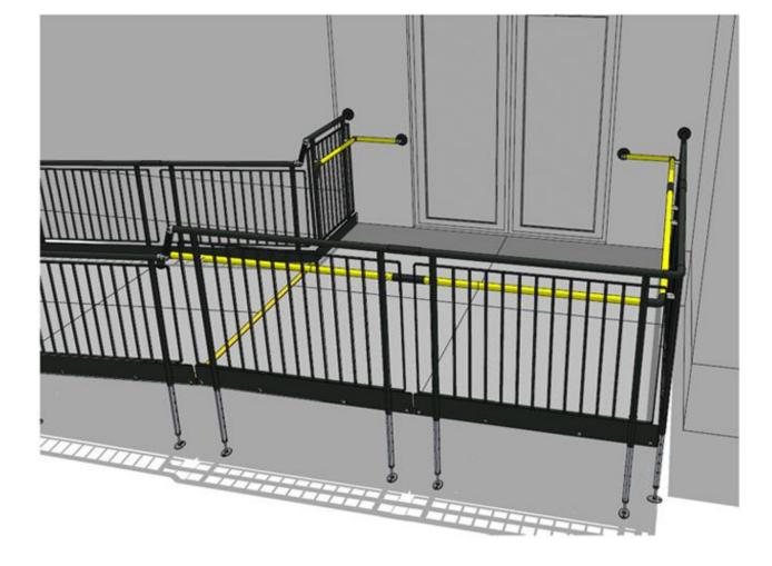
**END RESULT:** A fully compliant ramp featuring an extra-wide metal walkway was designed and successfully installed. This product boasts a secure loading capacity of over one ton!
