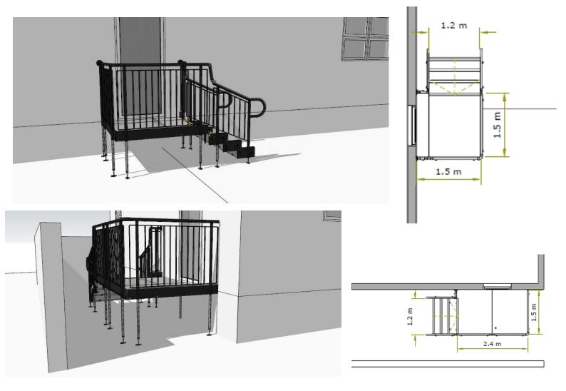
**END RESULT:** A fully compliant ramp was installed from the main entrance, along with step units from the other two doors.
