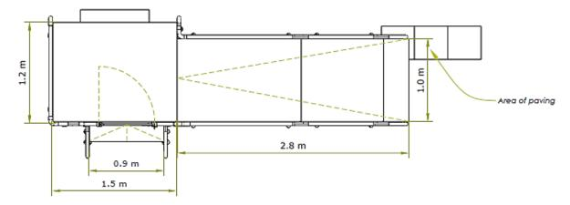
**END RESULT:** The ramp was installed within a few hours and included a 1:12 gradient.
